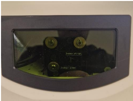
Illustration 8 Cross-hair Rotary Control
