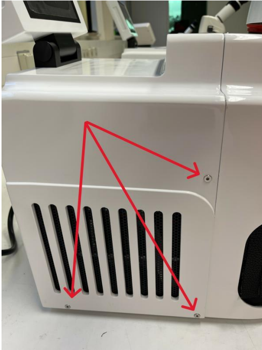
Illustration 19 Housing Screws sides and top
