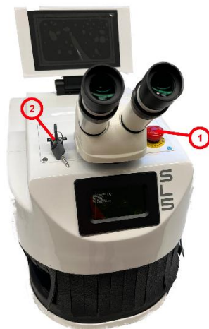
Illustration 1 1) Emergency Stop 2) Key Switch
